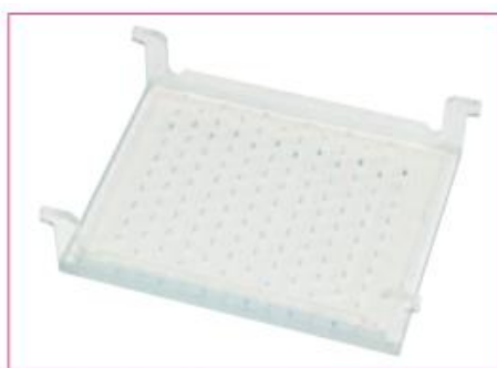
96 format UV tray with a cast gel
